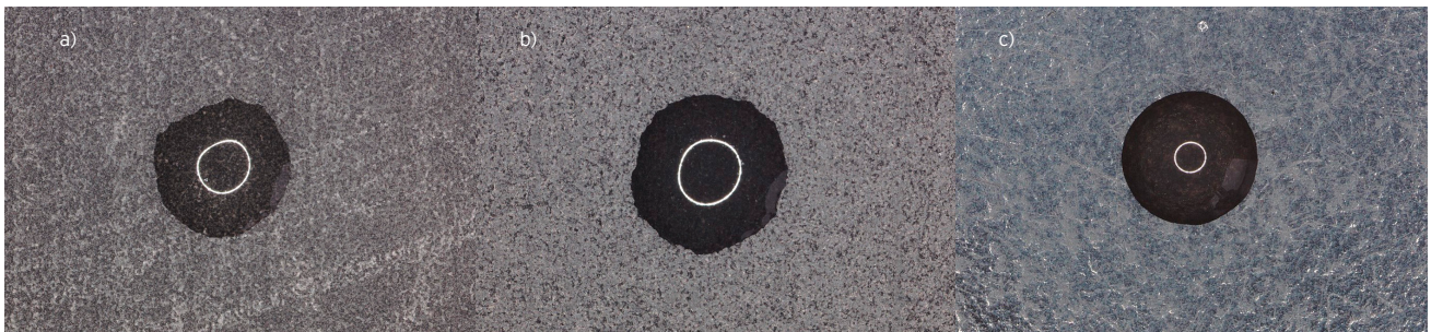
Figure 4: EOS PA 2200 parts with a water drop of 20 \mu L volume on differently treated surfaces. a) Water drop on colored EOS PA 2200 (r=4,5mm), b) on PSS treated and colored EOS PA 2200 (r=3,8mm), c) on VFS treated and colored EOS PA 2200 (r=2,7mm).
